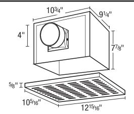
Acceptable for use over tub or shower when installed in a GFCI protected branch circuit.
